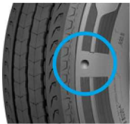
Sidewall Wear Indicators
