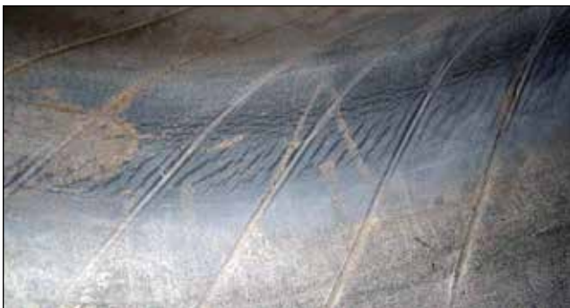
EFFECT: Inner Liner Marbling - Creasing CAUSE: Underinflation
