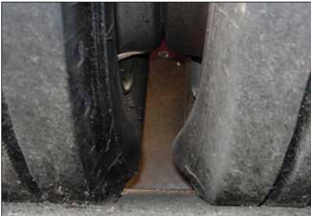
Underinflation in a dual configuration overloads the properly inflated tire. Both tires must be inspected.
