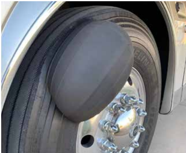
EFFECT: Inner liner damage CAUSE: Malfunctioned run-flat/bead lock device
